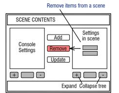
**Remove items from a Scene** Highlight items in the right hand window to remove from the Scene. To remove everything highlight Select All. Then touch the Remove button in the centre of the screen.
